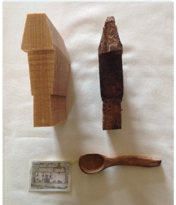
The new and old wooden teeth from the Barony Mill pictured above with a hand carved spoon by Anne Mathieson recycled from an old tooth.
